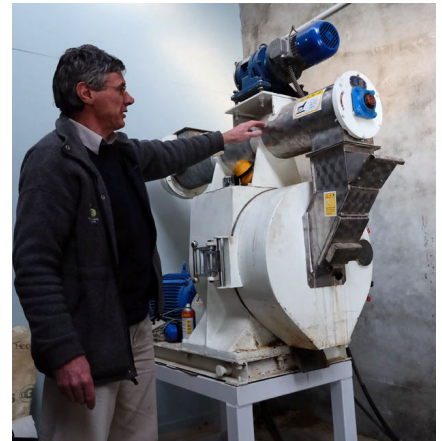
Malcolm Thomas with the small soon-to-be replaced pelletiser.
